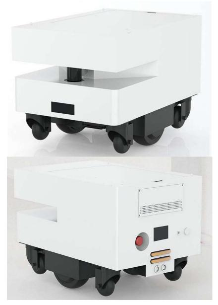
CaddyRanger is a light-duty general-purpose robot platform with a built-in high-performance navigation and positioning system. It comprises hardware such as LiDAR sensors and 3D and visual cameras. It has an open SDK platform and provides API interfaces. Users can carry different applications and expand according to actual needs. Suitable for commercial occasions such as shopping malls, hospitals, and restaurants.
