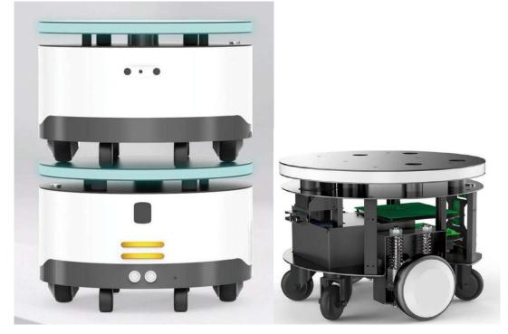
CaddyWheel is a light-duty general-purpose robot platform with a built-in high-performance navigation and positioning system. It comprises hardware such as LiDAR sensors and 3D and visual cameras. It has an open SDK platform and provides API interfaces. Users can carry different applications and expand according to actual needs—easier to maneuver, suitable for narrow paths in restaurants and similar settings.
