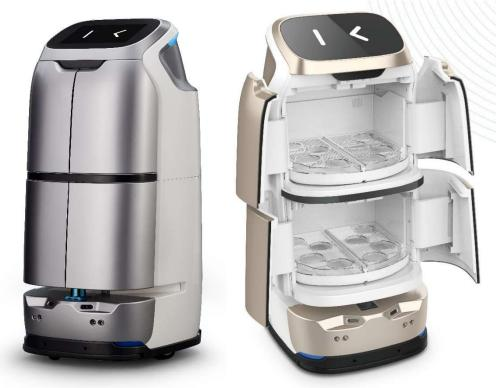
CaddyBot B3 does secure deliveries. The door is locked during the transportation. Upon arriving at the destination, a reminder voice will be announced. The door will be opened and picked up through passcode. The elevator module is available for multi-floor usage.
