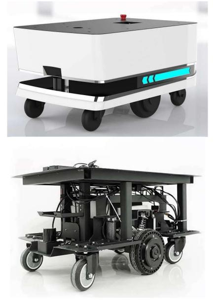
Caddyator is an extensible general-purpose robot platform with a built-in high-performance navigation and positioning system. It comprises core hardware such as LiDAR sensors, 3D and visual cameras. It has an open SDK platform and provides API interfaces. Users can carry different applications and expand according to actual needs. Extremely strong, suitable for commercial occasions such as shopping malls, hospitals, and restaurants.
