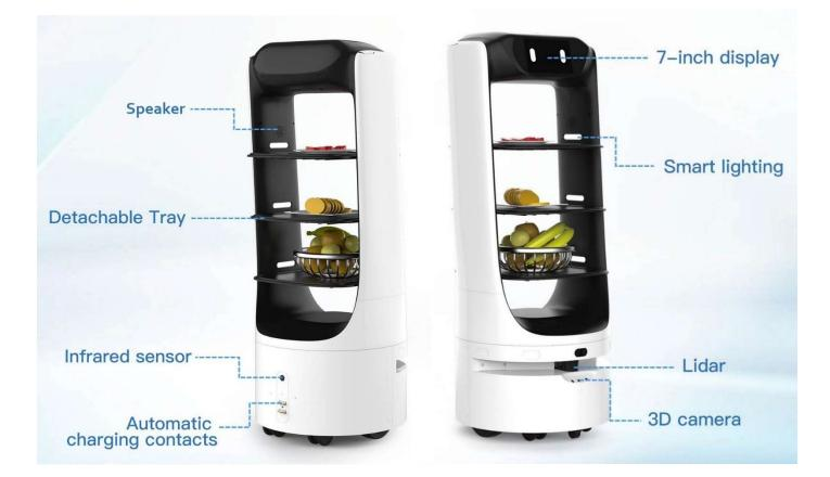
CaddyBot B1 is equipped with our leading autonomous scheduling system, which can automatically plan paths, high-precision navigation, positioning, autonomous obstacle avoidance, and automatic recharging. It is widely used in catering establishments such as hotels and restaurants.
