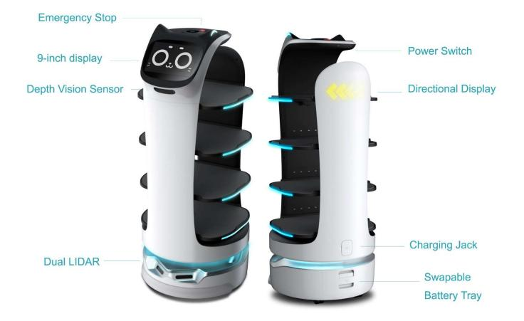
CaddyBot B2 food delivery robot is equipped with industry's first dual SLAM navigation solution, multi-machine collaboration, and autonomous obstacle avoidance. With its superlative trafficability, high-precision navigation and positioning, compact environment can be easily navigated.
