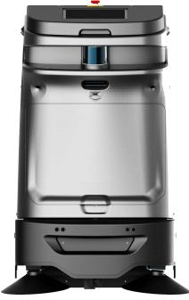
The M4/SP50 excels in picking up all types of debris, no matter how large or small. The robot is equipped with smart sensing technology and cutting-edge 3D lidar, that can recognize various types of debris on the floor and adjust its suction power accordingly. The robot is equipped with a powerful motor, with a maximum suction power of up to 25kPa.
